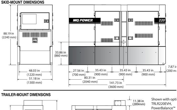
Stabilizer Jacks, MQ POWER 220 IC. 116.78 in Spare Tire, (2966 mm) Storage Box, 105.4 in (2677 mm) ▫▦▦ and Grab Handle 110 89 in 212.9 in (2261 mm) (5408 mm)
